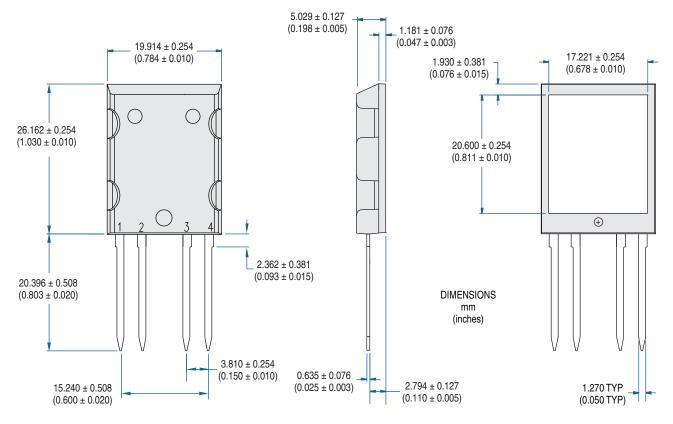
NOTE: Back-side heat sink meets  $2500V_{rms}$  isolation to the pins.
